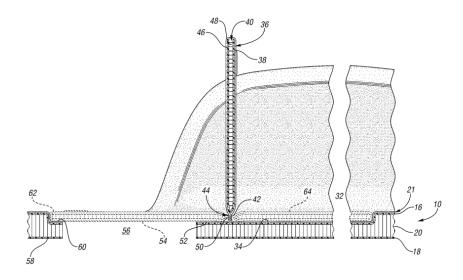
The specification discloses that hinged panel 10 is typically manufactured from a stack of material including "first and second reinforced thermoplastic skins 16 and 18, respectively, a thermoplastic cellular core 20 disposed between the skins 16 and 18 and a top layer of a substantially continuous covering layer generally indicated at 21." *Id.* at col. 4 ll. 35–42.
